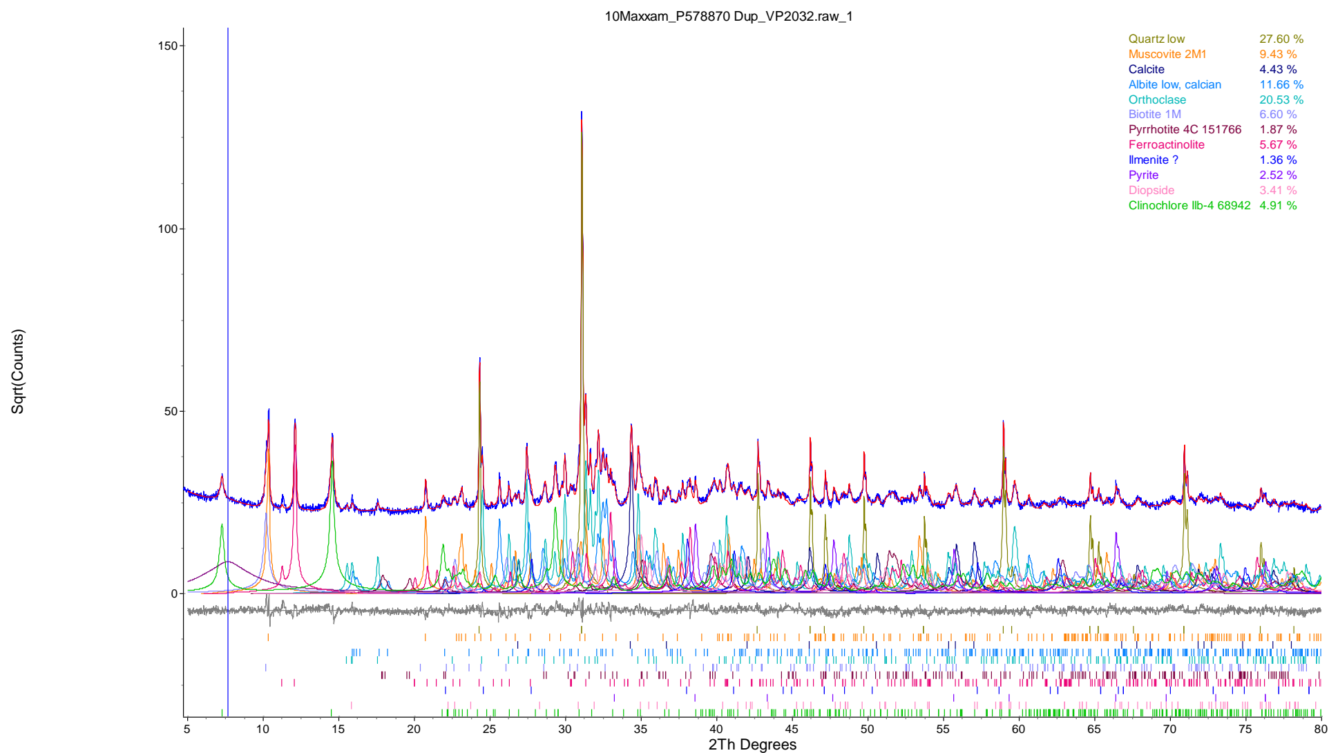
Figure 10. Rietveld refinement plot of sample Maxxam Analytics 10_P578870 Dup_VP2032 (blue line - observed intensity at each step; red line - calculated pattern; solid grey line below – difference between observed and calculated intensities; vertical bars - positions of all Bragg reflections). Coloured lines are individual diffraction patterns of all phases.
