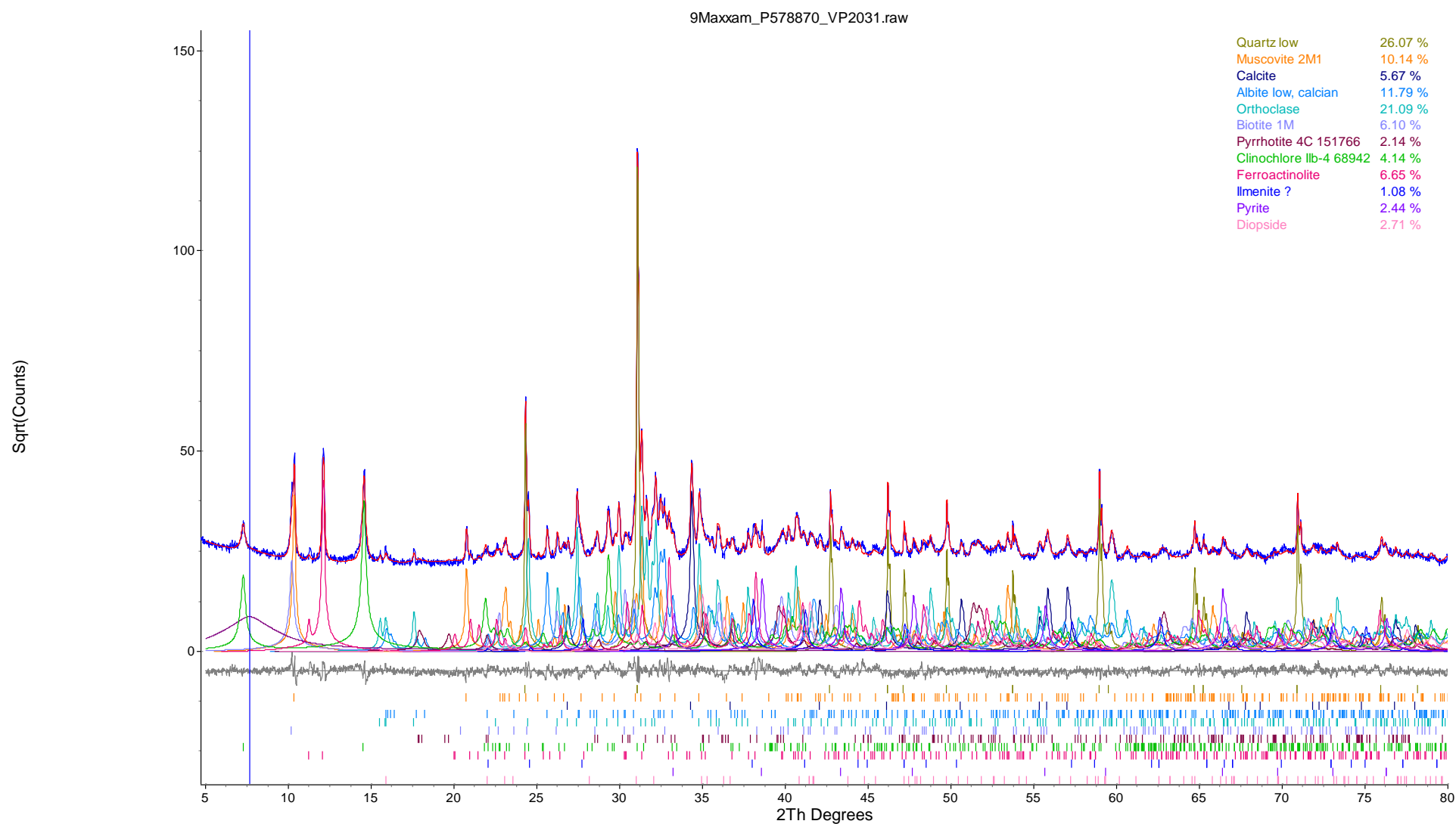
Figure 9. Rietveld refinement plot of sample Maxxam Analytics 9_P578870_VP2031 (blue line - observed intensity at each step; red line - calculated pattern; solid grey line below – difference between observed and calculated intensities; vertical bars - positions of all Bragg reflections). Coloured lines are individual diffraction patterns of all phases.
