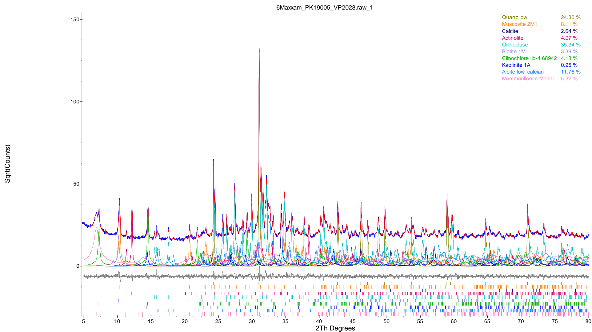
Figure 6. Rietveld refinement plot of sample Maxxam Analytics 6_PK19005_VP2028 (blue line - observed intensity at each step; red line - calculated pattern; solid grey line below – difference between observed and calculated intensities; vertical bars - positions of all Bragg reflections). Coloured lines are individual diffraction patterns of all phases.
