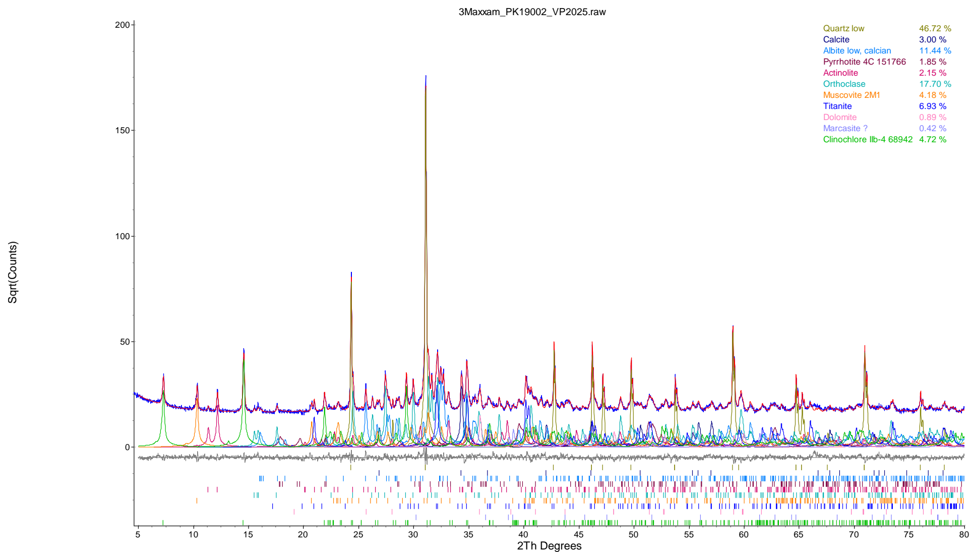
Figure 3. Rietveld refinement plot of sample Maxxam Analytics 3_PK19002_VP2025 (blue line - observed intensity at each step; red line - calculated pattern; solid grey line below – difference between observed and calculated intensities; vertical bars - positions of all Bragg reflections). Coloured lines are individual diffraction patterns of all phases.
