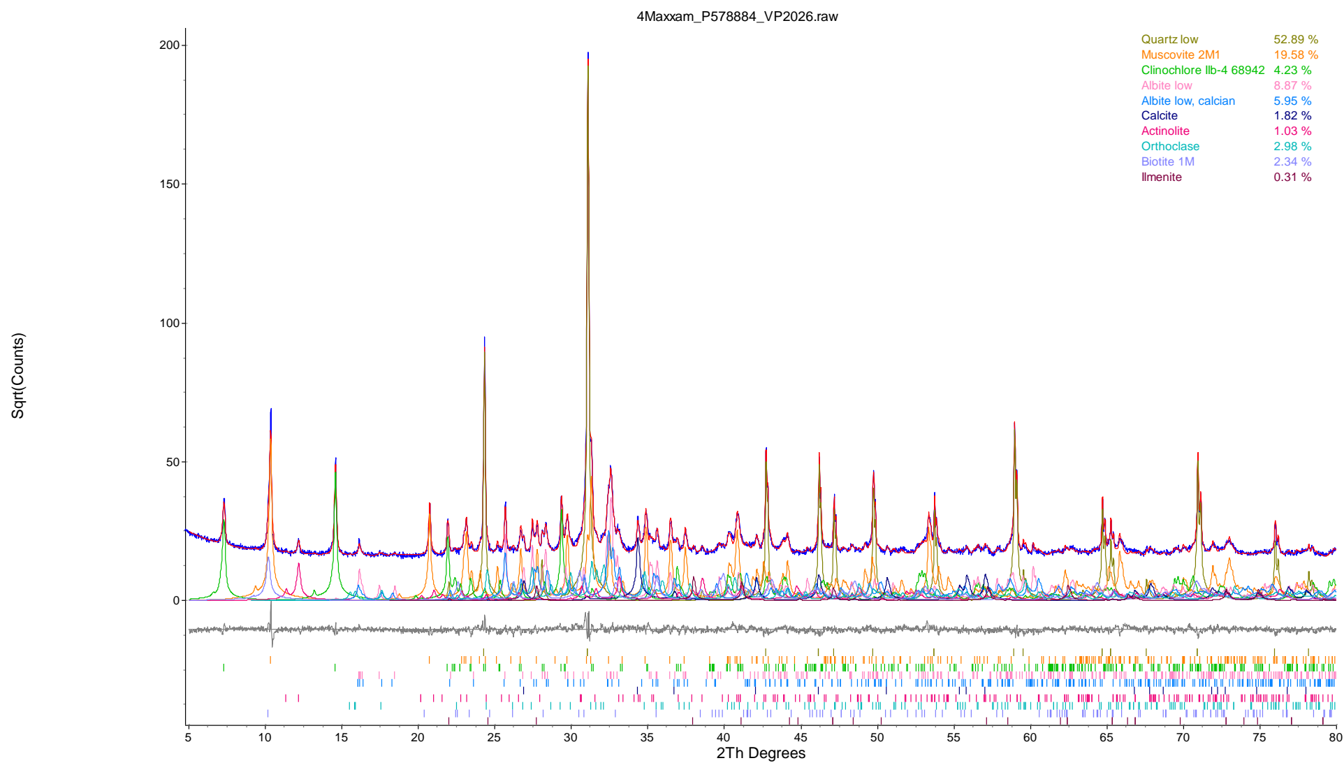
Figure 4. Rietveld refinement plot of sample Maxxam Analytics 4_P578884_VP2026 (blue line - observed intensity at each step; red line - calculated pattern; solid grey line below – difference between observed and calculated intensities; vertical bars - positions of all Bragg reflections). Coloured lines are individual diffraction patterns of all phases.
