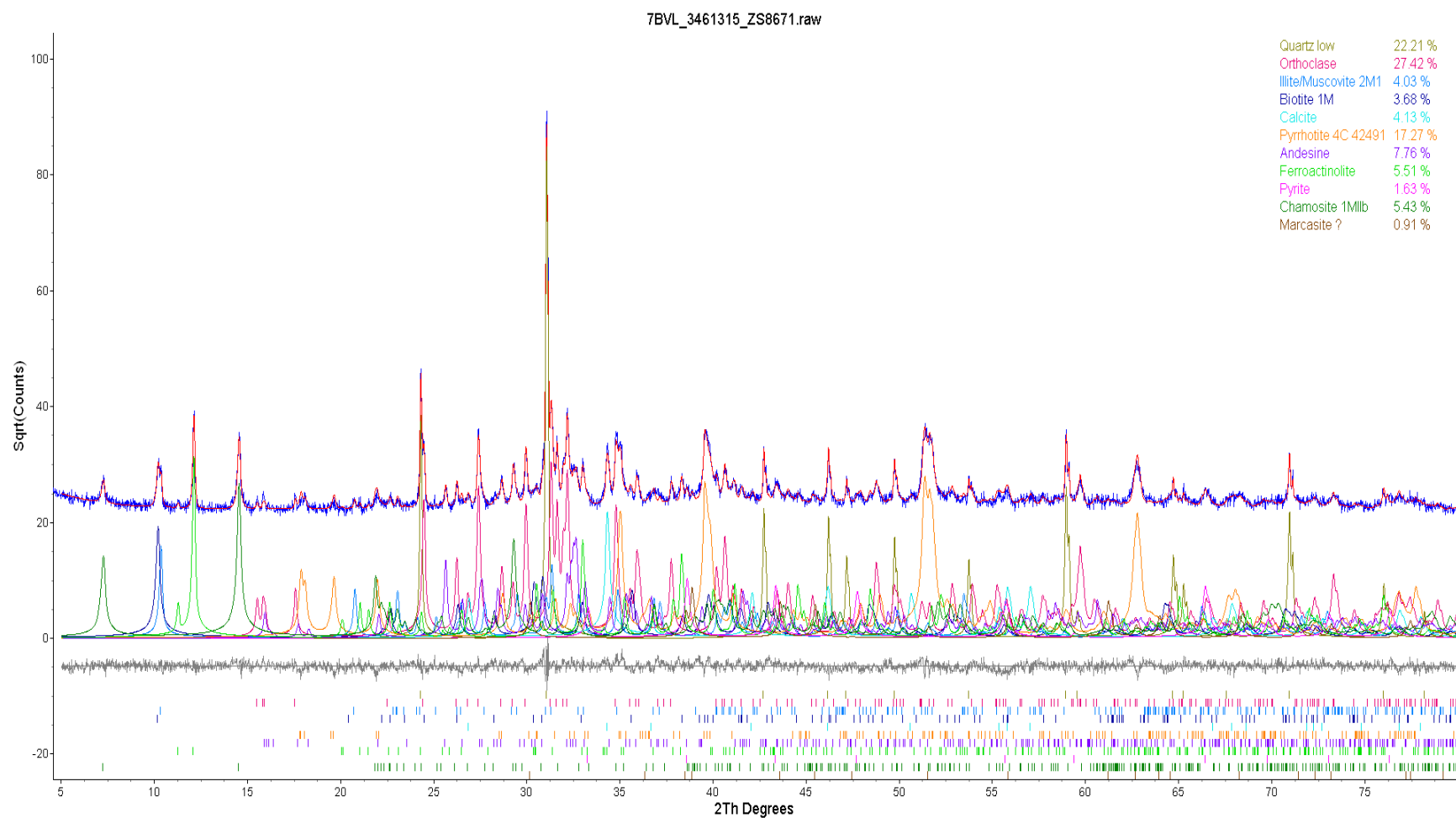
Figure 7. Rietveld refinement plot of sample BV Labs – #7: 3461315 (ZS8671) (blue line - observed intensity at each step; red line - calculated pattern; solid grey line below - difference between observed and calculated intensities; vertical bars - positions of all Bragg reflections). Coloured lines are individual diffraction patterns of all phases.
